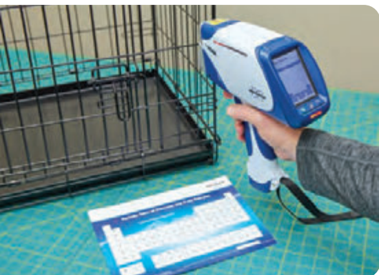
The XRF PMI gun analyzes the chemical composition of our metal products and verifies that our quality and safety standards are consistently met.
