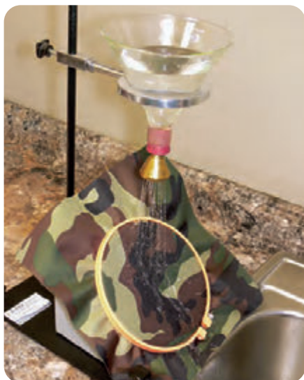
The Water Repellency Test measures the resistance of fabrics to wetting.
