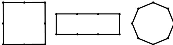
3. Connect the two ends with the snaps as shown in picture. For best results, place snaps at top and bottom between the two closely spaced wires, and space the remaining two snaps evenly along the middle wires.
